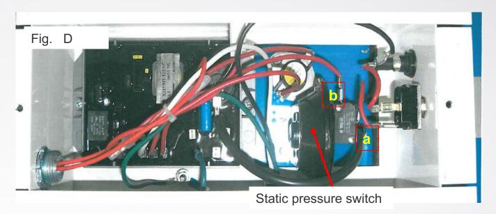
3. If there is voltage at "b" (Fig. D) then test for 120V at L1 on your control board. If there is voltage at L1 but not V1, the control board is defective ad must be replaced
