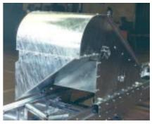
fixed control unit (with a 0,37 gear motor) and a return pulley. For the other series of machines, advancement is obtained by a gear motor mounted on board the tripper itself.
