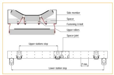
The following card records the main manufacturing specifications of the upright supports for the various series of conveyors. The feed rollers, due to a special profile of the side
