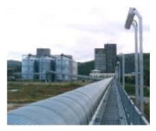
For a wharf installation, for pickup by the dock discharge towers, the upper cover has two flaps that can be opened to allow advancement of the inlet hopper. It is produced with a rubberised belt resting on a suitable supporting tubular structure and reinforced with elements in shaped sheet metal.
